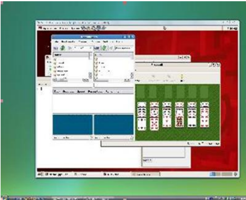
Fig 1. A remote X desktop displayed with LIVE on a local Windows Vista desktop
